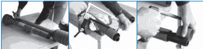
Figure 5 - Adjusting the length of the P.T.O shaft to the proper dimension for the tractor
