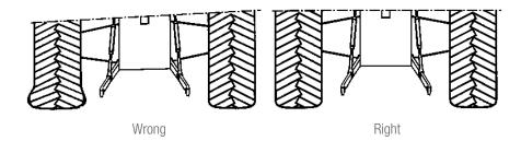
• Right and left link arms of the tractor must be adjusted to equal height from the ground.
