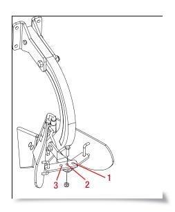
• The channel width setting is adjusted using fasteners by matching the holes 1,2 or 3 on the sheet metal shown in the figure. The channel width can vary between 34 cm and 46 cm.
