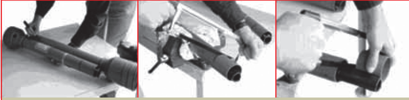
Figure 11 / Adjusting the length of the P.T.O shaft to the proper dimension for the tractor.
