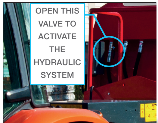
Figure 17 - Hydraulic system valve
