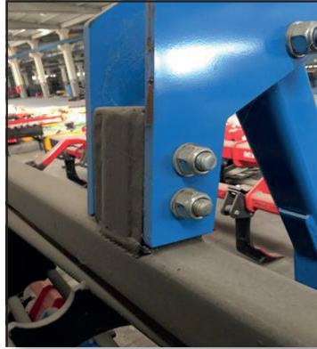
Figure 9 Roller Dismantling Bolt
